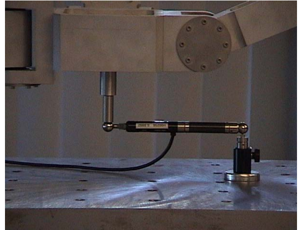
Fig. 6. Calibration experiment using a ball-bar.
